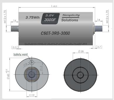
21. The maximum torque for threaded terminal is 12 Nm.
